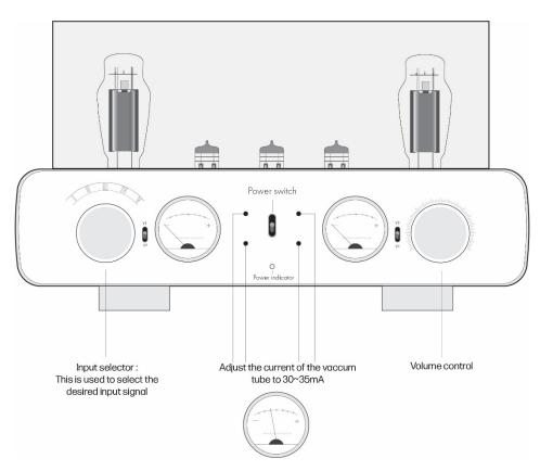
**Warm tips**: MELODY company reminds you not to blindly pursue perfect sound quality, 24 hours a day. This method is not suitable for vacuum tube amplifier. Because the service life of the electronic tube is only 2000 hours, equivalent to 84 days
